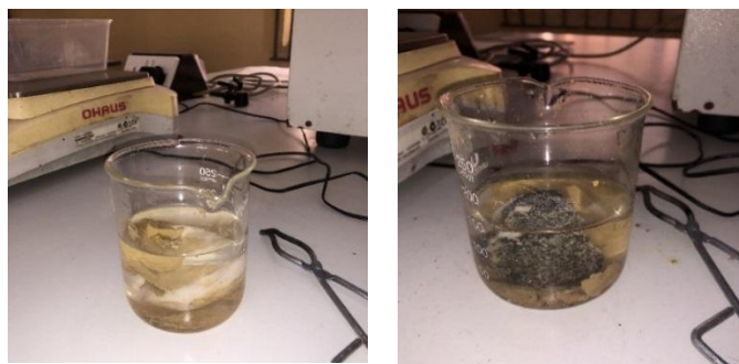
Figure 2: Rock sample in acid blend concentration for dissolution
