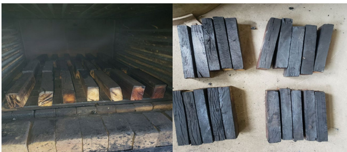
Plate 4: Post-Test Specimen Showing Char Layer
