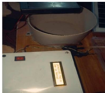
Figure 9. Assembled FEWS prototype during laboratory simulation. The LCD displays real-time water level and zone status; alert LEDs confirm threshold crossing; the relay and solenoid valve occupy the lower section
