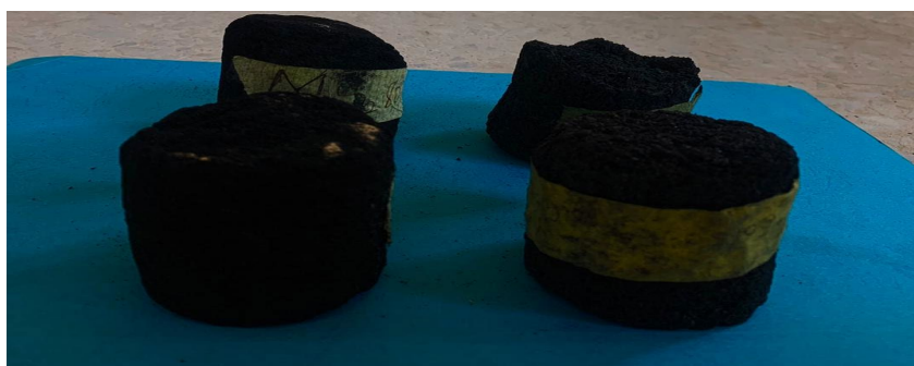
Figure 2: Carbonized cashew nut shell briquettes
