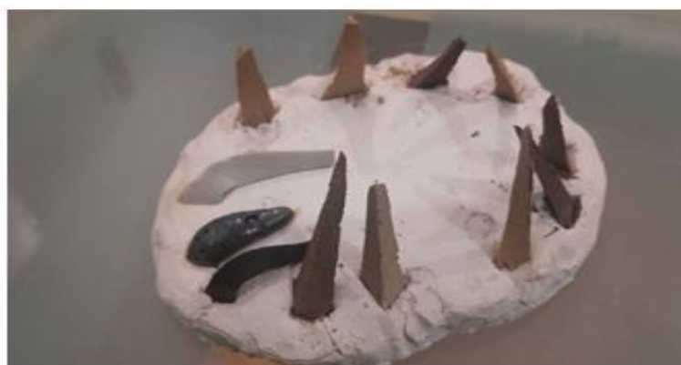
Figure 11: Showing standard cones squatting while test samples remain standing
