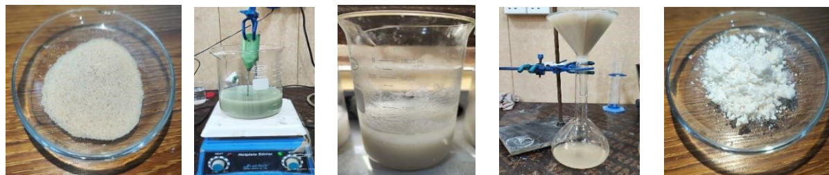
Figure 3: Silica production stages of nano silica (SiO 2 ) by sol-gel.
