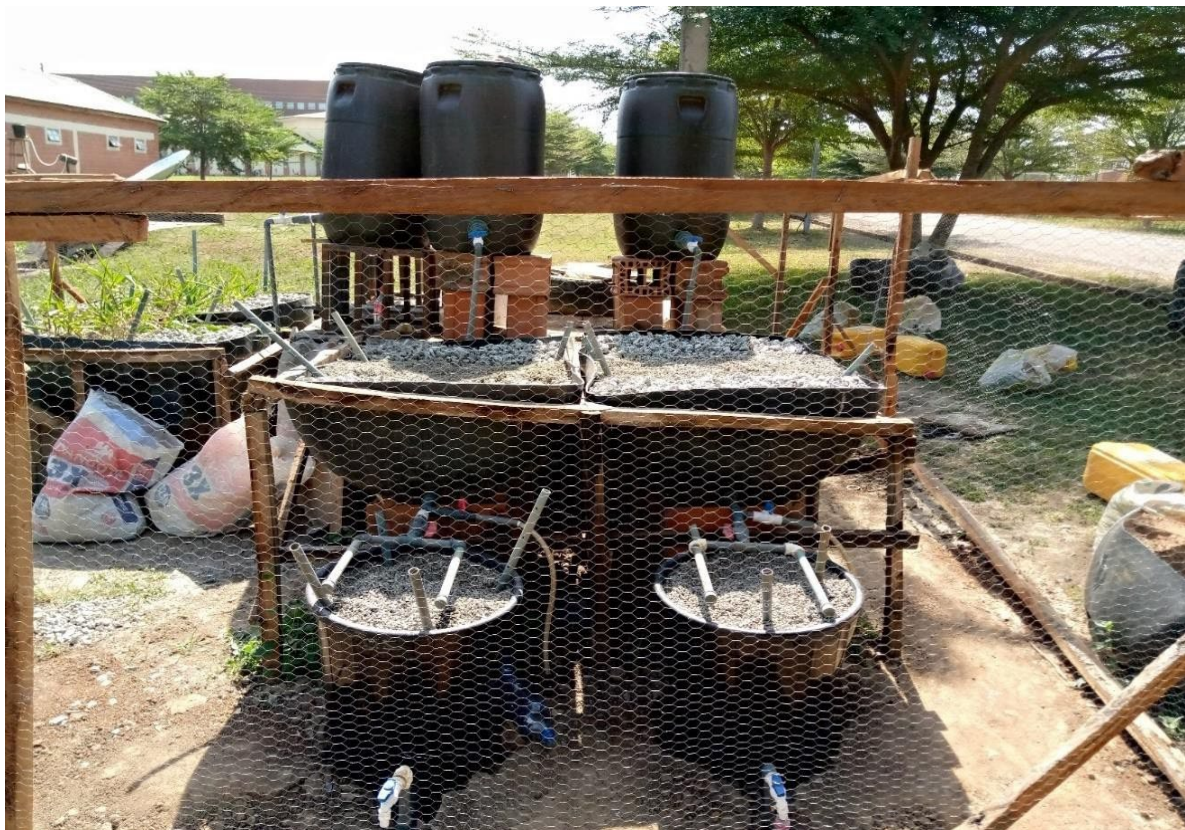
Plate 1: Set-up of Unplanted hybrid constructed wetlands
