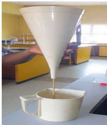
Figure 4: Marsh funnel used in measuring the rate at which the test fluid drains
