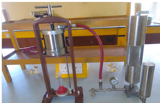
Figure 5: Dead weight filter press used to determine the filtration properties of the mud
