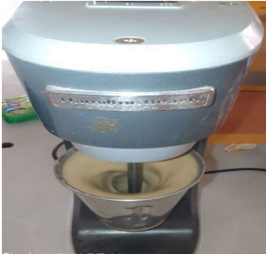
Figure 3: Hamilton beach stirrer used in formulating mud
