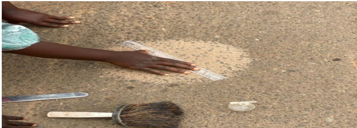
Figure 1: Measurement of surface texture depth by sand patch test
