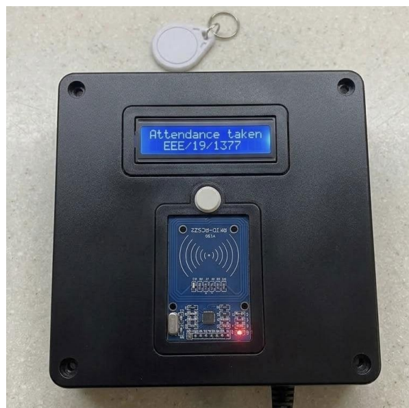
Figure 5: The RFID-based Smart Attendance System Display Showing 'Attendance Taken' and the matric number recorded
