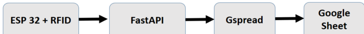
Figure 6: Data flow of the IoT-based smart attendance system from the ESP32 and RFID module to the Google Sheets cloud storage.
