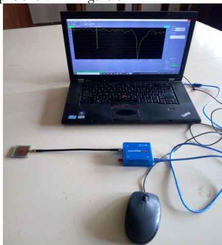
Figure 8: Antenna performance measurement setup
