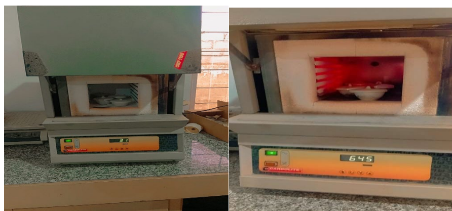
Figure 3: Muffle furnace (Carbolite CWF11/5, 1/98/51) used for the determination of ash content and volatile matter with the support of ceramic dishes
