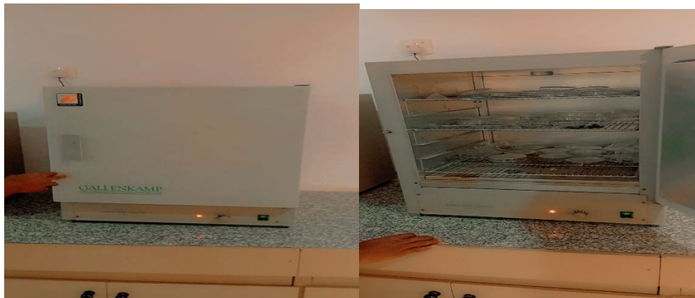
Figure 2: Electric oven (Gallenkamp OHF097.XX.1.5) used for moisture determination
