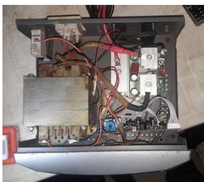
(a) Inverter (top view)
