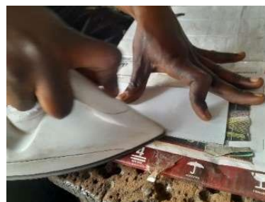
(b) Transfer of design by heat
