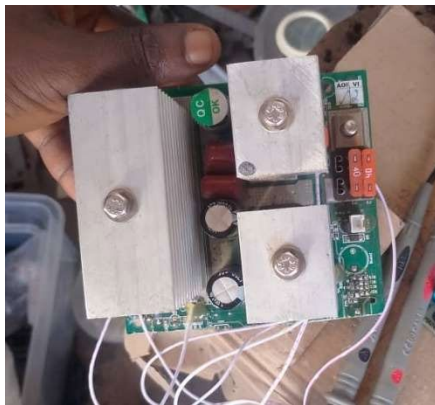
(a) MOSFET Board (Top view)
