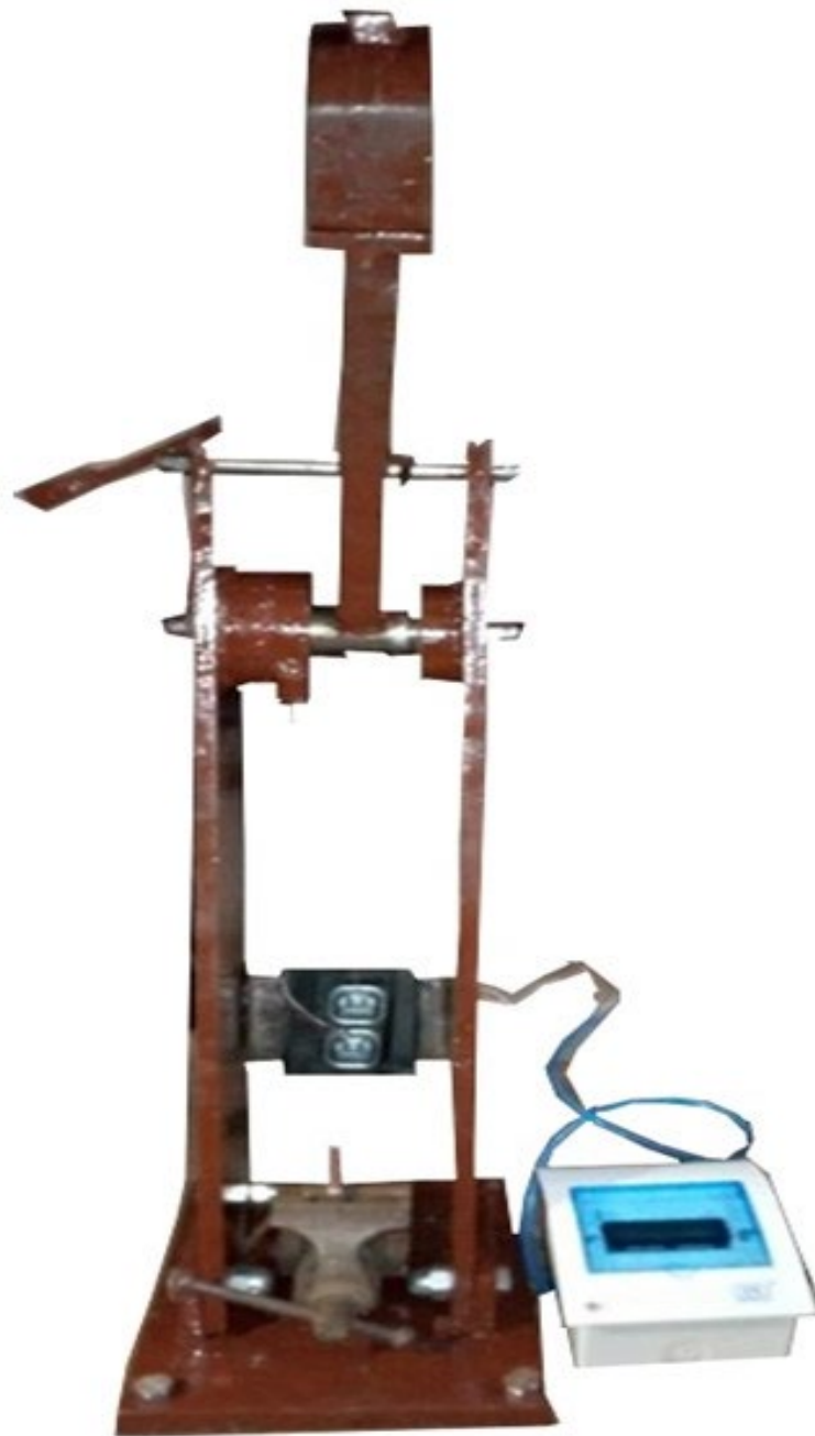
Figure 8: Impact fracture tester experimental set- up
