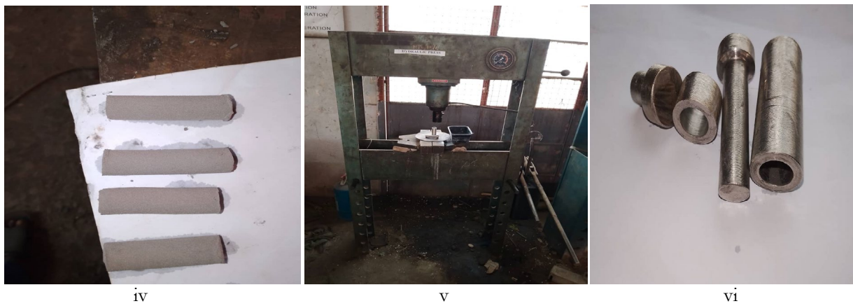
Figure 1: (a) ethylene glycol (binder), and Ti6Al4V alloy powder, and hydroxyapatite (b) Ti6Al4V powder being weighed on a weighing balance (c) 15mm diameter x 15mm green samples produced (d) 15mm diameter x 60mm green samples produced (e) hydraulic press (f) prepared moulds for samples
