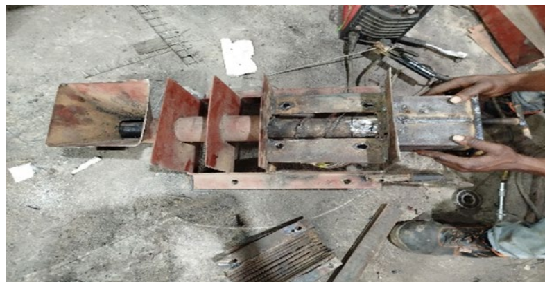
Plate 3: Fabrication and Fittings of Stopper
