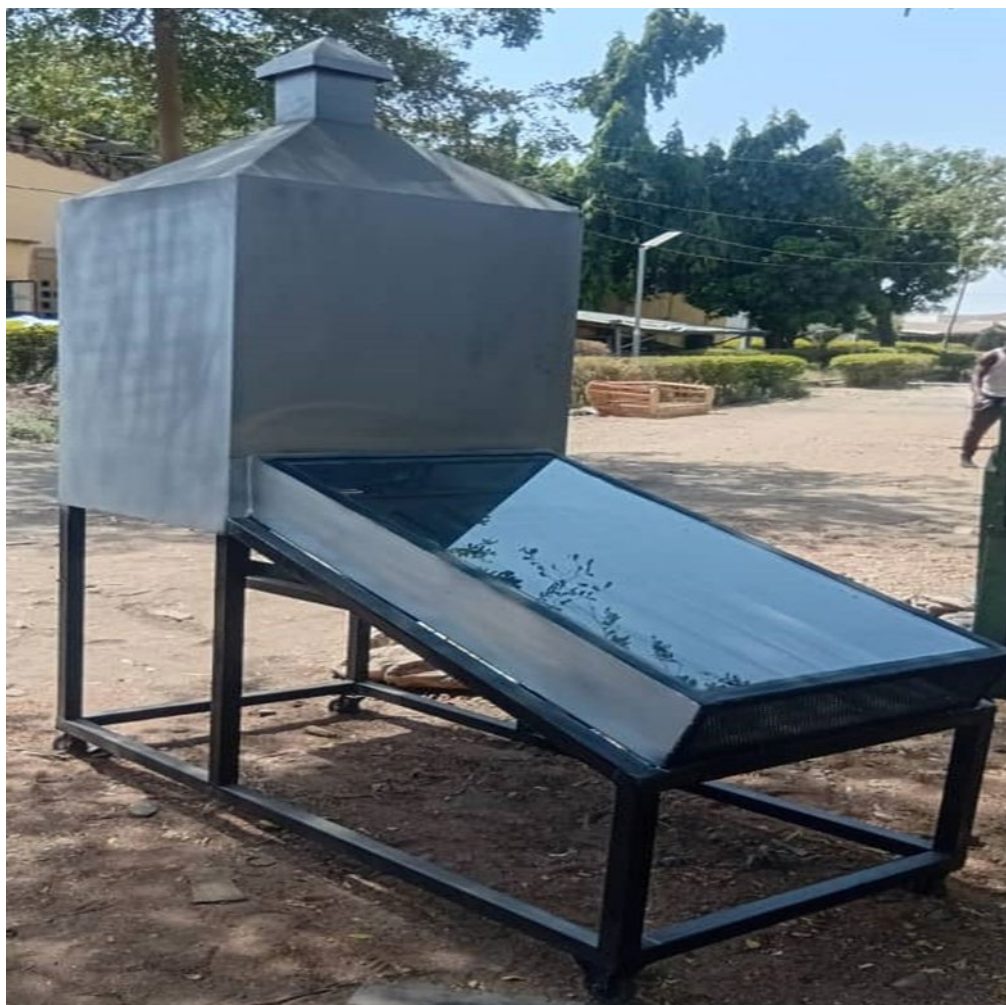
Plate 2: Rear view of the constructed dryer
