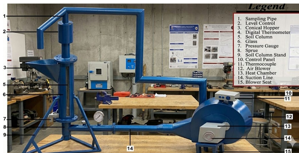
Figure 3: Pilot scale soil column air stripping system
