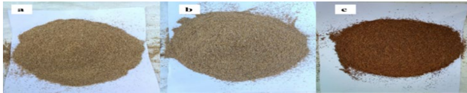
Plate II: (a) Groundnut Shells (b) Groundnut Melon Shells (c) Groundnut Shea nut Shells
